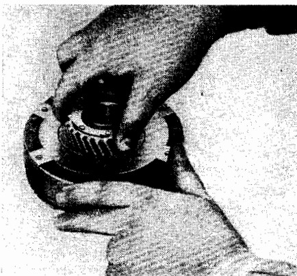
Fig. 28. Clearance between clutch driver – disk with friction lining
