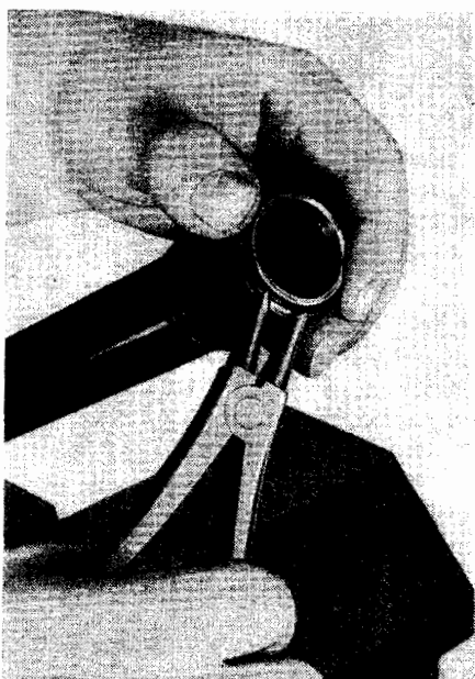
Fig. 103 Loosening the lower circlip
