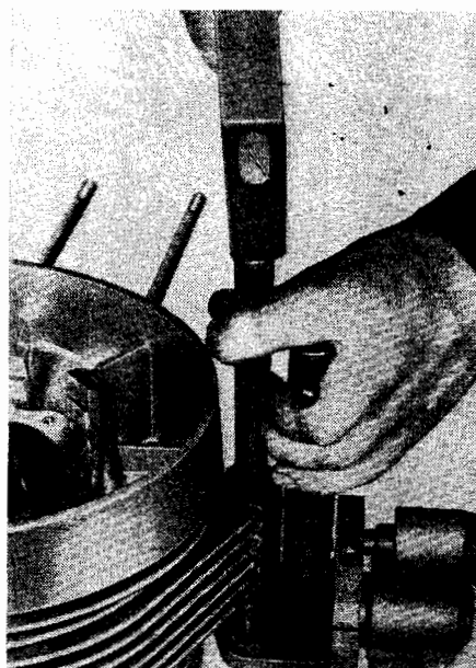
Fig. 59 Driving the fitting sleeve in place
